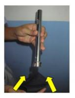
Use a piece of cloth to hold the stator as the teeth are sharp and can cut you!
