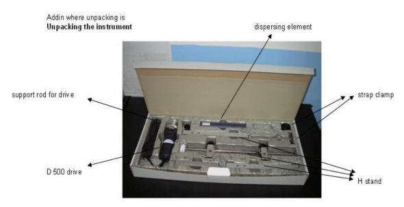
Please unpack the instrument carefully and inspect the unit, the tools and the stand for damage. It is important that any damage during transport is noted at the time of unpacking.
